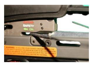
6) Pointing in a safe direction, take the safety off and squeeze the trigger. You will hear a click. Your serving is now being supported by the Crossbow Decocker. Holding the crossbow by the foregrip with one hand, and pointing in a safe direction, unscrew the T knob with your dominant hand until the string and serving are in the defused/neutral position. Unscrew the T knob just slightly more, slide back 1/2", tighten, and lift off.
