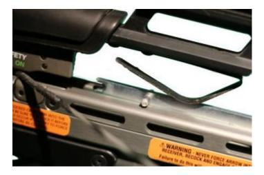
4) Raise up the ball end and slide the U-brace (T knob upright) over and down, resting on the barrel between the riser and cables
